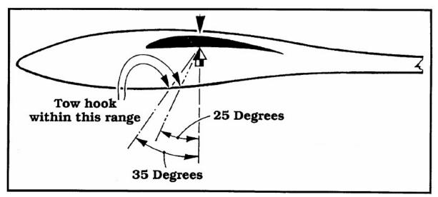
O.K., let's assume we don't know where to install our tow hook, so let's start by installing the tow hook at 30 degrees, in front of the C.G. On launch, while watching the model go up, do you see only the trailing edge of the wing or can you see the top of the wing?
